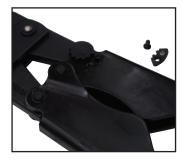
I. Remove the screw and the locking plate.
