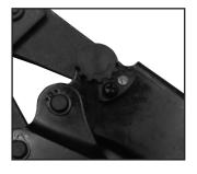
3. Replace the locking plate and the screw.
